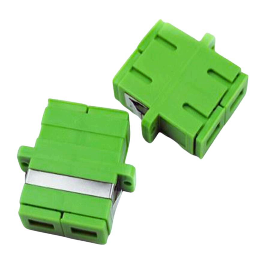
The VertexConnect Duplex SM SC/APC-SC fiber optic cable connector ensures minimal signal loss, making it ideal for FTTH, LAN, MAN, CATV, and PON distribution. Designed for reliable installation in patch-panels, it supports single-mode fiber with SC/APC connectors, operating effectively between -25°C and +70°C.
